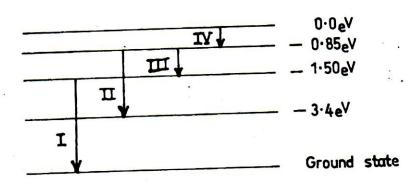
The diagram above illustrates some energy levels in an atom of hydrogen. Which of the transitions I - IV will produce an absorption spectra line in the hydrogen emission spectrum?
