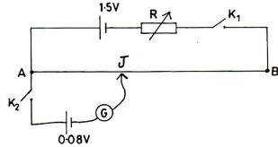
The diagram above illustrates a uniform potentiometer wire **AB** of length 100 cm and resistance 2  $\Omega$ . A cell of e.m.f. 1.5 V and a variable resistor **R** are connected in series with **AB**. If **R** = 4  $\Omega$  and the key  $K_1$  is closed, calculate the
