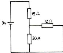
Using the Kirchhoff's rule, determine the current through each resistor in the diagram above.
