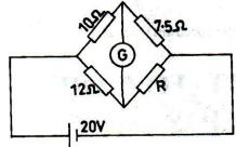
Use the circuit diagram above to determine the value of R at null deflection.
